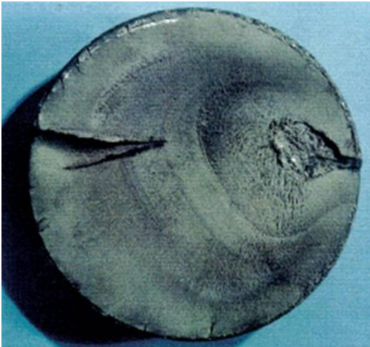
Fatigue Fracture with Beachmarks
